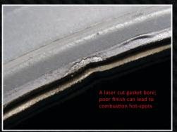
Demand a STOPPER LAYER; a precision fold around the cylinder bore creating a load point for superior combustion sealing
