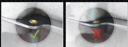
NO PART of any rivet should be compressed between cylinder head and block
