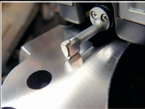
Diamond tipped stylus measuring block surface
